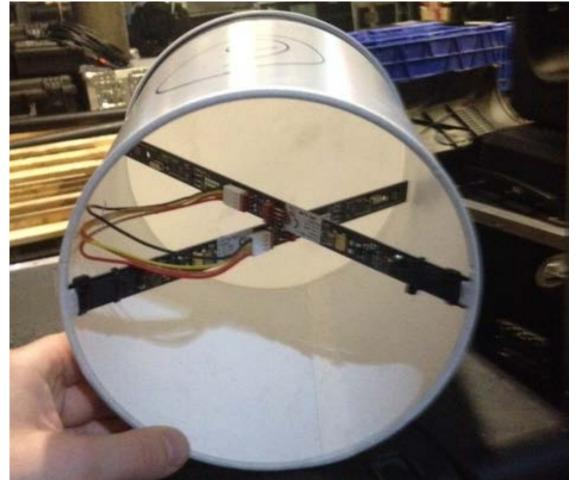
Above The aluminum pipes already fitted with Schnick-Schnack-Systems technology before the stage was built.
